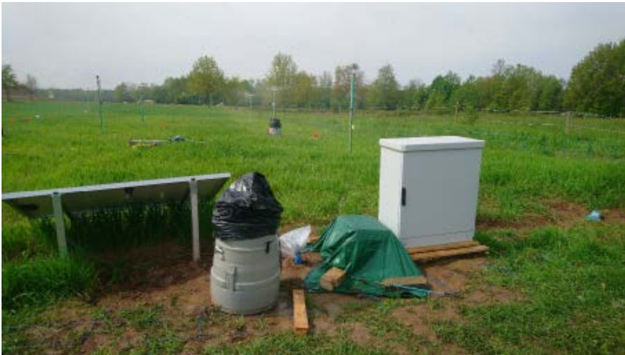
Figure 3: The experimental agricultural field in Germany, showing the sprinklers simulating rainfall events in the back as well as solar panel for powering the instruments, such as the autosampler and the Multispecies Freshwater Biomonitor, MFB, and the battery storage station (from left to right)
