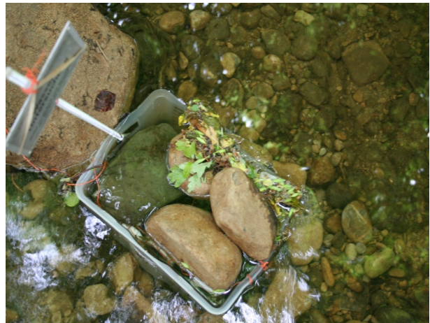
Figure 1. Experimental setup: Exposure of a basket with 5 plexiglass cages in the Hornbach at the downstream site. Photo A. Gerhardt.
